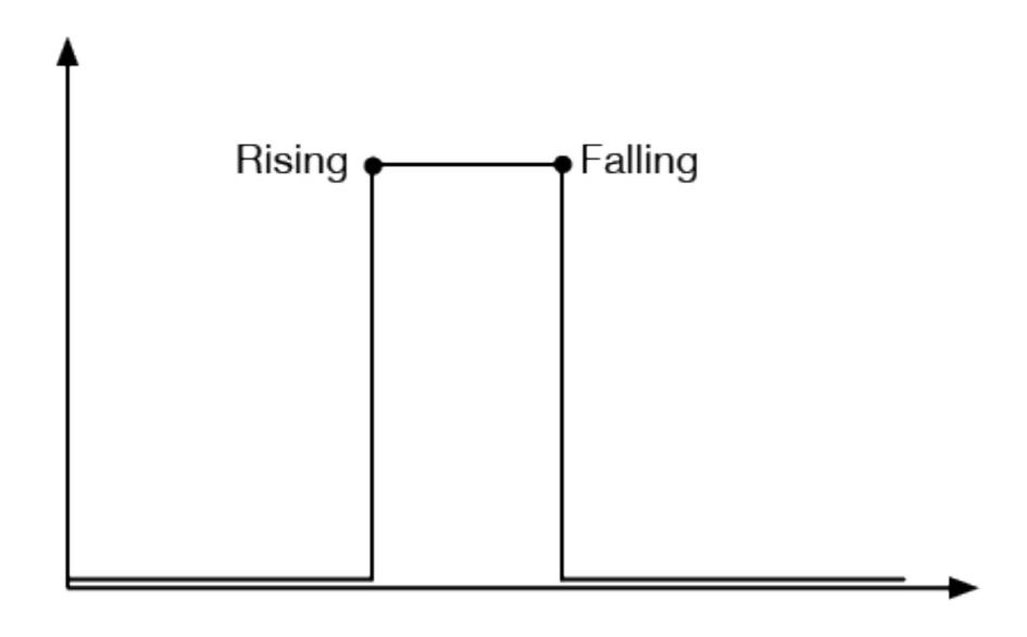
DIGITAL SENSORS CHANGE FROM HIGH VOLTAGE TO LOW AND VICE VERSA. THE CHANGE FROM LOW VOLTAGE TO HIGH IS CALLED THE RISING EDGE, & THE CHANGE FROM HIGH VOLTAGE TO LOW IS CALLED THE FALLING EDGE.
